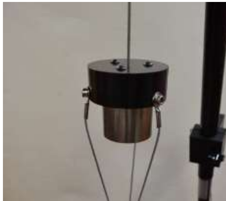
Photo 3 – Connection of test fixture to tripod
