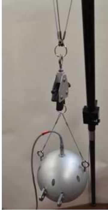
Photo 2 – Head form suspended from reference test fixture
