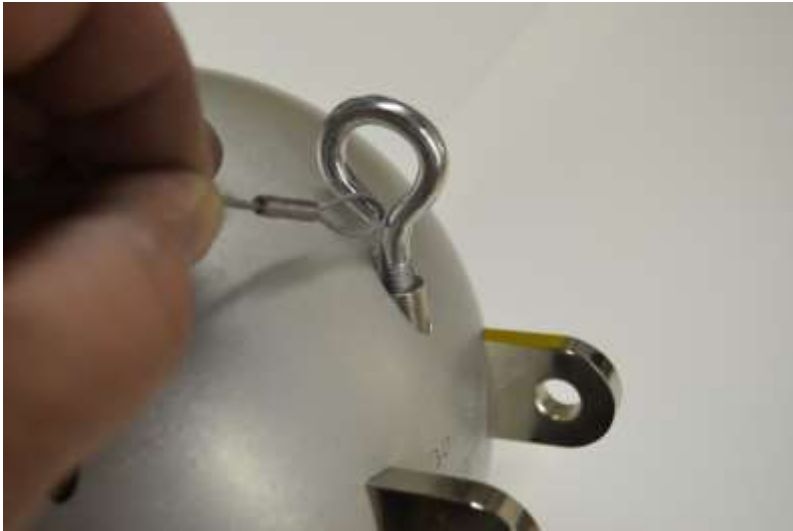
Photo 4- Connecting wire rope lanyard to eye head
